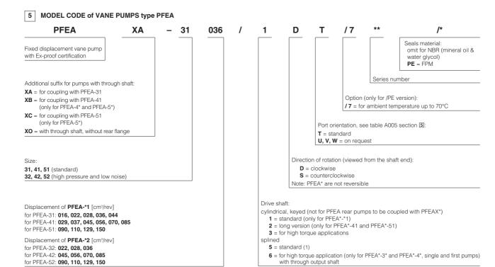
1) Shaft type 5 has to be selected for PFEA rear pumps to be coupled with PFEAX\* first pumps
