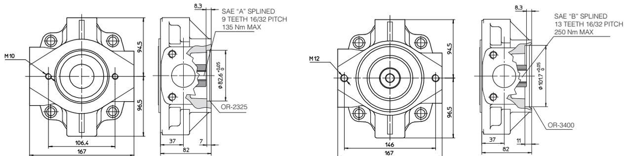
Drawing shows pumps with clockwise rotation (option D): pumps with counterclockwise rotation (option S) will have inlet and outlet ports inverted
