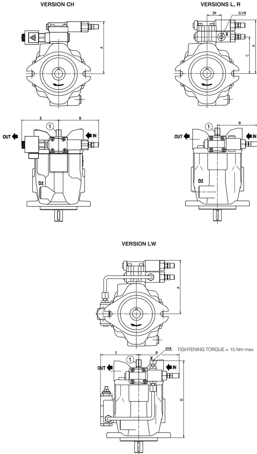
① = Regulation screw for max displacement. Adjustable range 50% to 100% of max displacement).
