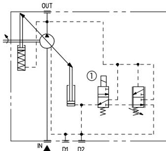
**CH Manual pressure compensator with venting**
