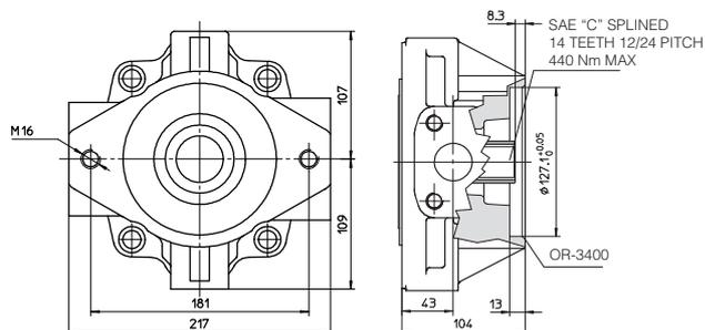
Drawing show pumps with clockwise rotation (option D); pumps with counterclockwise rotation (option S) will have inlet and outlet ports inverted
