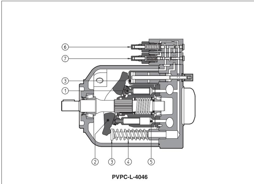
PVPC are variable displacement axial piston pumps for high pressure operation, with low noise level, suitable for hydraulic oils or synthetic fluids having similar lubricating characteristics.
