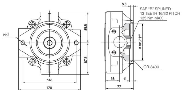
Drawing shows pumps with clockwise rotation (option D); pumps with counterclockwise rotation (option S) will have inlet and outlet ports inverted
