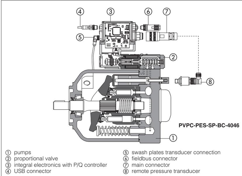
The variable displacement axial piston pumps type PVPC, can be supplied with advanced electrohydraulic proportional controls:
