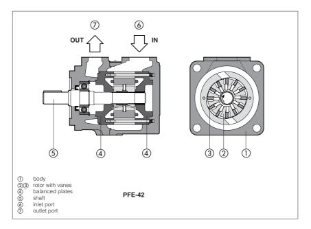
New PFE-\*2 are fixed displacement -twelve-vanes pumps 23, cartridge design with integral hydraulic balancing 4) for high pressure operation and long service life with further reduction of noise level compared with PFE-\*1.
