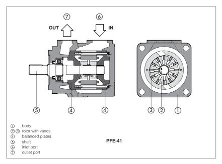
PFE-\*1 are fixed displacement-twelvevane pumps, ② ③ cartridge design with integral hydraulic balancing ④ for high pressure operation, long service life and low noise level.
